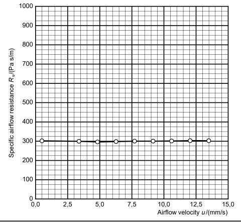
Specific airflow resistance  $R_s(0.5 \text{ mm/s}) = 295 \text{ Pa s/m}$
